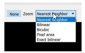
Selection of interpolation type is via the combobox next to the zoom button above the image.
