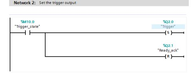
3. When the Ladder logic receives the trigger ACK-bit from the slave device, it resets the trigger bit.
