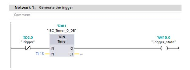
2. When the trigger pulse is generated, the Ladder logic sets the trigger bit, and resets the ready ACK-bit on the slave device.
