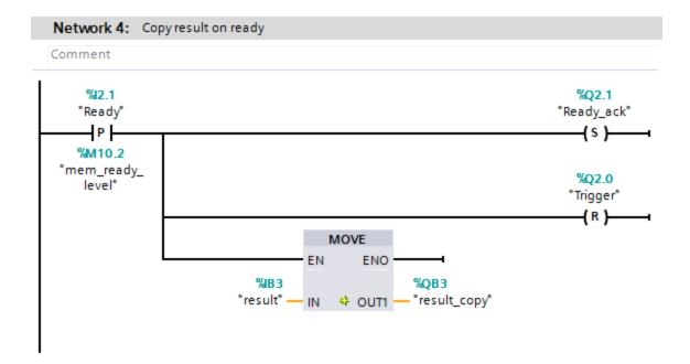
The following table contains the resulting sequence of the Ladder code.
