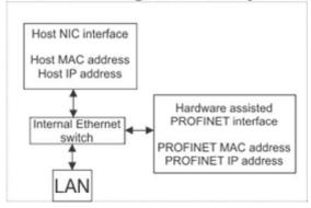
Both interfaces require a static IP address to be set. The static IP address of the hardware-assisted PROFINET interface must be compatible with the automation network. The Host NIC interface should also be set to a static IP address, otherwise the Auto-IP or DHCP modes might lead to the connection failing when the Host NIC interface attempts to discover a DHCP server or renegotiate its IP address.
