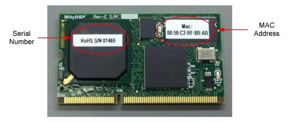
The serial number and MAC address of the MityDSP-XM SOM may be determined by the figure below.
