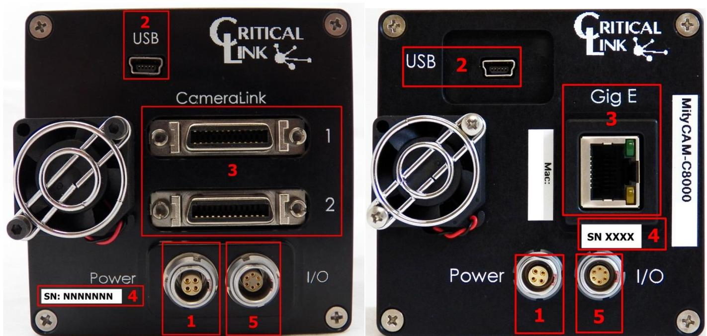
Figure 1 – MityCAM-C8000 Camera Link (Left) and Gigabit Ethernet (Right)
